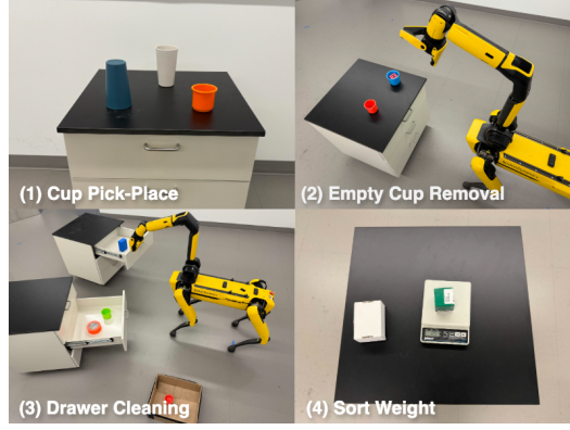
Figure 8.1: Example tasks demonstrating various uncertainty levels. (1) Cup Pick-Place: a fully observable tabletop manipulation task with multiple cups. (2) Empty Cup Removal: requires inspecting cups from above to determine if they are empty before removal. (3) Drawer Cleaning: involves opening drawers to discover and remove objects inside. (4) Sort Weight: requires weighing sealed boxes on a scale to identify and dispose of empty ones. These tasks demonstrate increasing complexity in information gathering, from fully observable scenarios to those requiring several strategic information-gathering steps.
